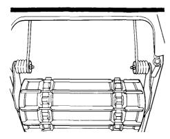
Track (M) S Lift the rear of the vehicle and support it off the ground so that the track is free to turn. With engine off, rotate track by
