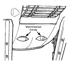
**Caution:** To keep efficiency of the cooling system, check that the belly pan ventilation holes are not blocked or obstructed.
