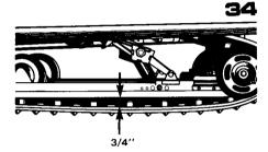
Track Tension (Slide Suspension) Lift rear of vehicle and support it off the ground. Allow slide to extend normally. A gap of 3/4" should exist between slider shoe and bottom inside of track. If track tension is too loose, the track will have a tendency to thump. Too much tension will result in power loss and excessive stresses on suspension components. If necessary to adjust, loosen or tighten adjuster bolts located on inner side of rear idler wheels.
