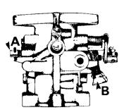
Low Speed Mixture Adjustment (A) With engine off, turn Low Speed Mixture Screw fully clockwise until closed. Then back off screw one (1) turn counterclockwise. Do not close screw too tightly as screw and/or screw seat can be damaged
